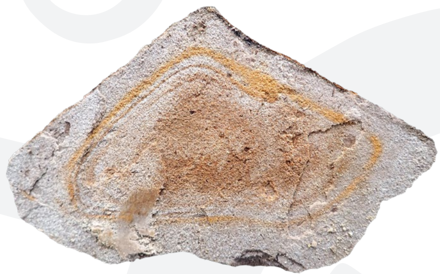
Rustringe Circular rust stains
